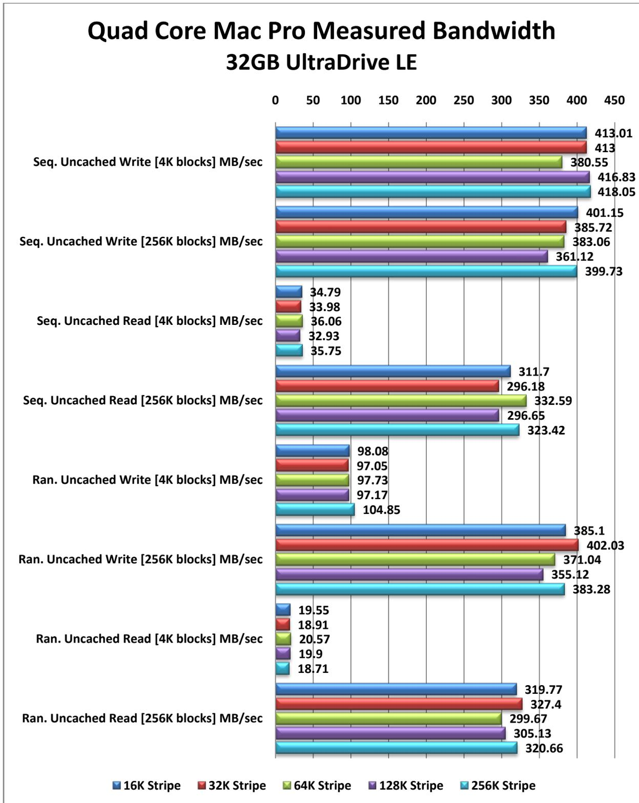
Figure 11: Mac Pro 32GB UltraDrive LE Stripe Test Measured Bandwidth
